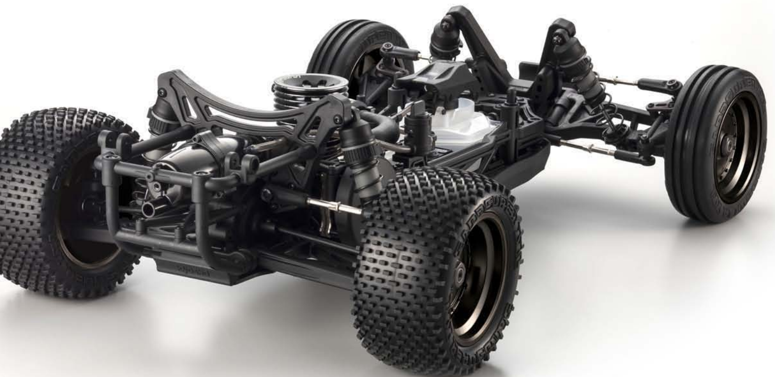
Resin shock stays are resilient under extreme punishment. Use of hard material eliminates unnecessary deflection. Increases effectiveness of suspension.
